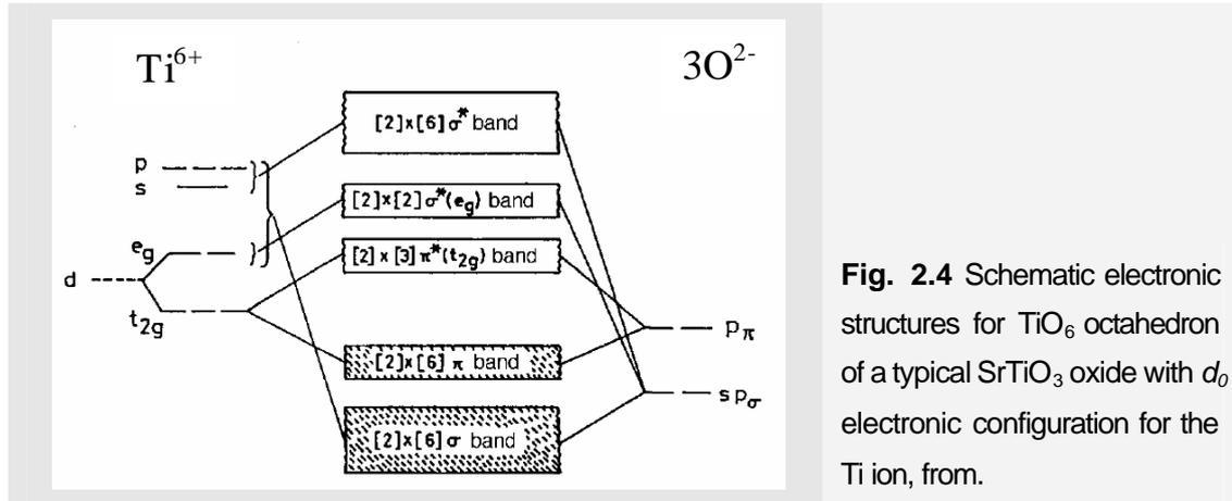
**Fig. 2.4** Schematic electronic structures for  $\text{TiO}_6$  octahedron of a typical  $\text{SrTiO}_3$  oxide with  $d_0$  electronic configuration for the Ti ion, from.
