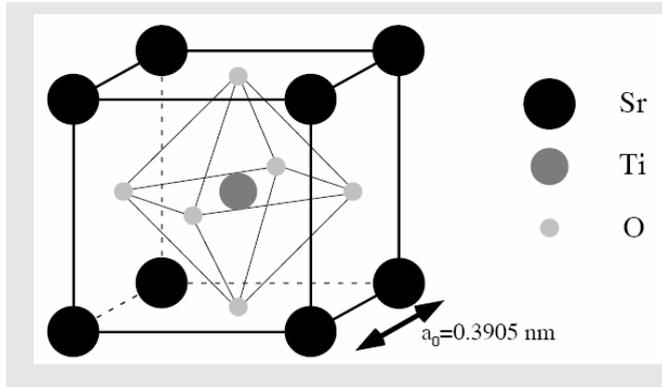
**Fig. 2.1** Atomic structure of SrTiO<sub>3</sub> at RT. The sizes of the spheres representing the atoms are arbitrary and are not related to atomic radii.
