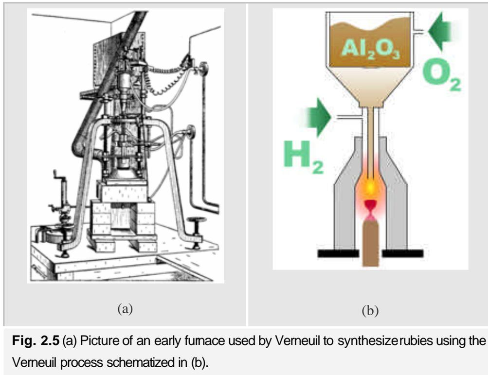
**Fig. 2.5** (a) Picture of an early furnace used by Verneuil to synthesize rubies using the Verneuil process schematized in (b).
