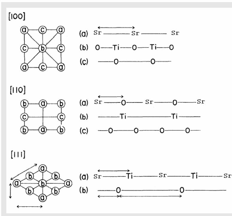
**Fig. 2.2** Atomic arrangements for the  $\langle 100 \rangle$ ,  $\langle 110 \rangle$  and  $\langle 111 \rangle$  axial directions in SrTiO<sub>3</sub>. The arrangements shown on the left are end views of the channels, and the letters refer to the individual rows shown on the right.
