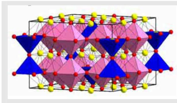
**Fig. 2.3** Ordering of oxygen vacancies in  $\text{SrFeO}_{2.875}$  ( $=\text{Sr}_8\text{Fe}_8\text{O}_{23}$ ). Fe ions are located in both square pyramids and in octahedral.
